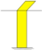
Yellow vertical stripes on the lock walls in front of the lock gates, extending from the water level to the lock platform and 1 m further on the lock platform itself.
